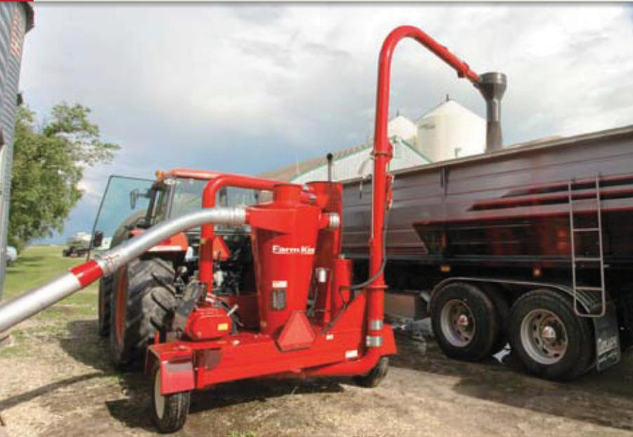
**Model 6640** The high vacuum suction carries the crop on a pillow of air and aids in cleaning out trash particles as the crop goes through the grain vac. The versatility of the grain vac hoses and cleanup wands allow the operator to access hard-to-reach areas for superior cleaning. The optional self-contained hydraulics allow the grain vac to be fully operational without using the hydraulic ports of the tractor.
